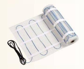
**FHM:** Floor Heating Mats comprise of flexible, robust fiber-glass mats that carry thin heating elements uniformly fixed on it. These elements are provided with primary fluoropolymer insulation, metal shielding and sheathing of PVC or fluoropolymer.
