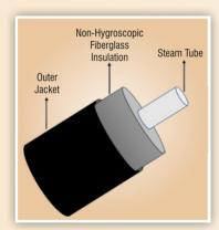
The pre-insulated tube is used to transport high temperature gas or liquid samples from its source to destination. On most occasions this is used to provide personnel safety from high temperature surfaces or to prevent sample temperature loss during transport.
